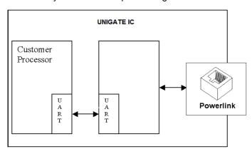
After the RS232-driver has been replaced by the UNIGATE® IC, Powerlink is available at an RJ45-socket.
