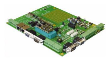
The required UNIGATE® IC / ICs are ordered separately. The required voltage (5V or 3.3V, depending on the version) can be adjusted. An RS232-interface or a USB-connection is available for the connection to the PC (Debug-interface).
