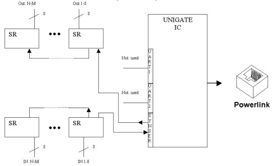
Here only the synchronous serial interface is used, the asynchronous serial interface is basically of no account. If you want to program the script in your completed application, then the use of a connector for the asynchronous interface is recommended. With it you can carry out the ISP-programming.
