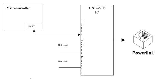
The  ${\sf UNIGATE}^{\it \&}$  IC independently processes the communication with the customer's device via the TTL-interface.
