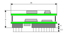
The pins of UNIGATE® IC - Interbus are arranged with a grid spacing of 2.54 mm.
