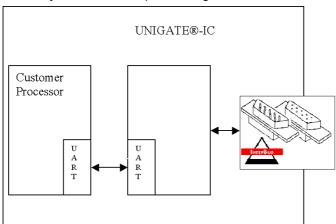
After the RS232-driver has been replaced by the UNIGATE® IC, the Interbus<sup>1</sup> is available at the 9-pol. D-sub-socket.
