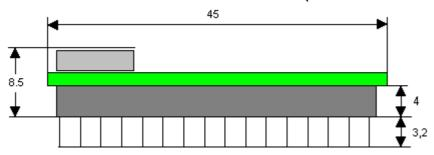
The pins of UNIGATE® IC - Interbus are arranged with a grid spacing of 2.54 mm.
