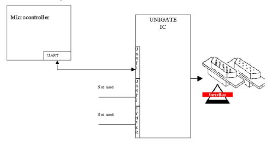
The UNIGATE® IC independently processes the communication with the customer's device via the TTL-interface.
