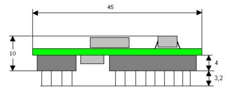
The pins of UNIGATE® IC - Ethernet are arranged with a grid spacing of 2.54 mm.
