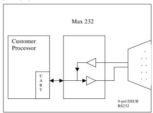
Your device, which on the whole is supposed to be assembled as shown above, will now be modified in a way that the Ethernet is available at the 9-pol. socket. However, a hardware redesign is necessary in order to keep the assignment in standard form.
