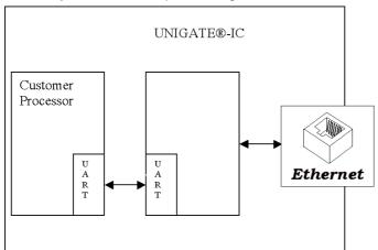
After the RS232-driver has been replaced by the UNIGATE® IC, Ethernet is available at an R.I45-socket
