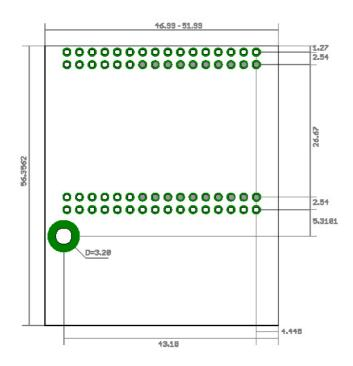
The pins of the UNIGATE<sup>®</sup> FC - EtherNet/IP 2Port are arranged 2, 54 mm in the contact pitch.
