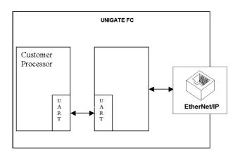
After the RS232-driver has been replaced by the UNIGATE<sup>®</sup> FC, EtherNet/IP is available at an RJ45-socket.
