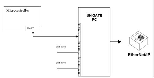
The UNIGATE<sup>®</sup> FC independently processes the communication with the customer's device via the TTL-interface.
