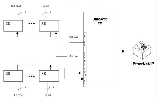
Version 2: Use of UNIGATE<sup>®</sup> FC for digital or analog I/O-modules
