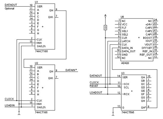
The following circuit diagram is an example for how shift register components can be connected to the FC.
