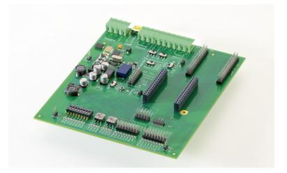
The required UNIGATE<sup>®</sup> FCs are ordered separately. An RS232-interface or a USB-connection is available for the connection to the PC (Debug-interface).
