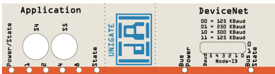
Front panel: Rotary switches, DIP-switch and LEDs
