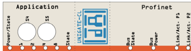
Picture 2: Front panel: Rotary switches and LEDs
