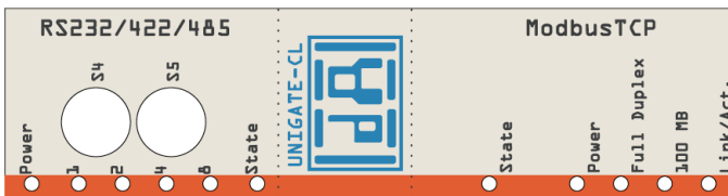
Bild 2: Front panel: Rotary switches and LEDs (from hard.-rev. B on)
