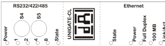
Bild 2: Front panel: Rotary switches and LEDs (from hard.-rev. B on)
