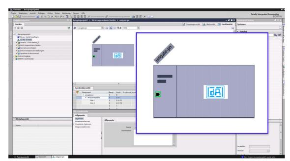
I/O modules can then be added automatically via the catalog by double-clicking.
