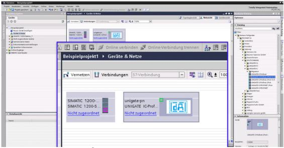
Depending on the UNIGATE<sup>®</sup> device, I/O modules may have to be added. For this, the UNIGATE<sup>®</sup> device must first be marked with a double click so that the "device overview" is opened.
