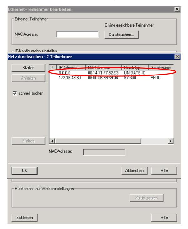
The MAC address of the selected device is now displayed in the following window. Enter the device name that was previously assigned in the properties under "Assign device name".
