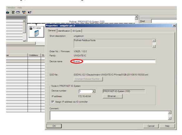
After the device has been inserted into the project, the device name must be stored. This must match the current device name that was entered in the properties window. Only then can the device be recognized by the master.
