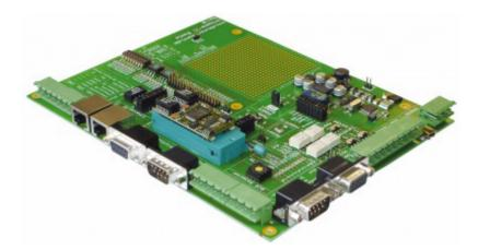
The required UNIGATE<sup>®</sup> IC2 / ICs are ordered separately. The required voltage (5V or 3.3V, depending on the version) can be adjusted. An RS232-interface or a USB-connection is available for the connection to the PC (Debug-interface).
